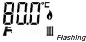
Radiator Symbol Radiator Circuit Temperature
